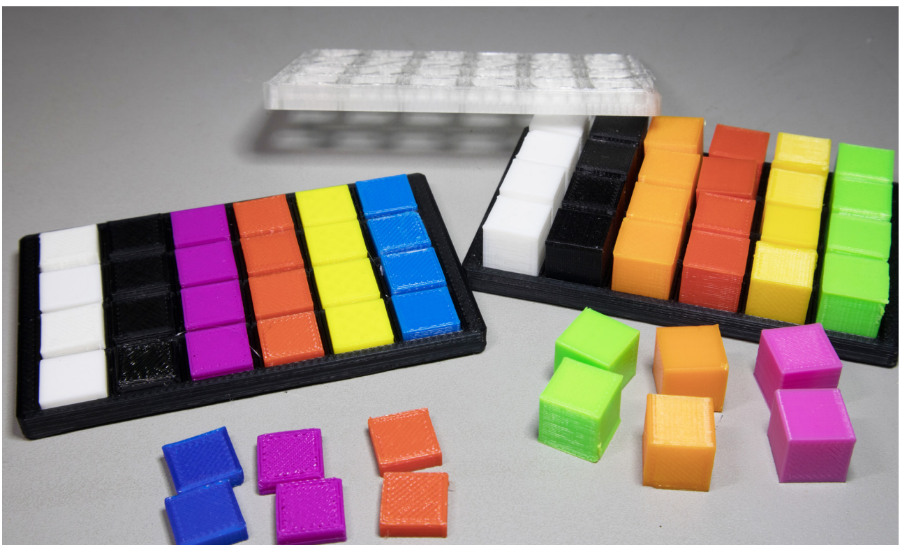
Figure 1. Photo of the Ryerson-Wilhelm Imaging Research 3D-printed color test target showing versions with 1-cm cubes (top) and 1×1×0.5-cm square tiles (bottom). The color cubes or flat, square tiles can be 3D-printed and exposed to high-intensity indoor illumination, placed in outdoor daylight weathering tests, subjected to ozone resistance tests, or long-term (Arrhenius) dark stability tests. During the course of the tests, the samples are measured spectrophotometrically with a multispectral camera and image analysis software is used to quantify fading, color balance shifts, and other degradation.
