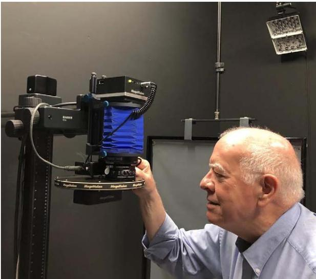
**Figure 8.** Henry Wilhelm adjusts the MegaVision EV Multispectral Camera. The EV is a spectral imaging system that employs a 50-megapixel monochrome CCD with a configurable LED array of up to 19 narrow-band LEDs (visible in upper right corner: UV 365, 385, and 400 nm; Visible 420, 450, 470, 505, 530, 560, 595, 615, 630, and 655 nm; and IR 700, 735, 780, 850, 940, and 1050 nm) in place of white light as the illuminant.
