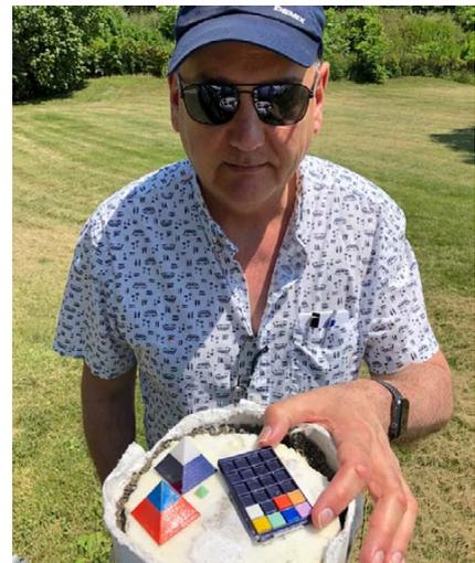
Figure 4. Richard Adams with a 3D color target in the outdoor location where it was exposed to sunlight, rain, and snow for one year.
