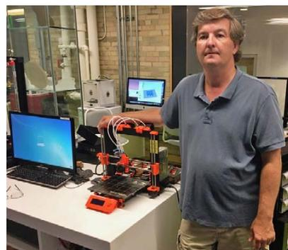
**Figure 2.** Jeremy Littler works in Ryerson University's Digital Fabrication Lab (Digital FabLab) with the Prusa MK2 3D printer that printed the 3D color target. For this project, PLA filaments of various colors were used to print the test target color patches.
