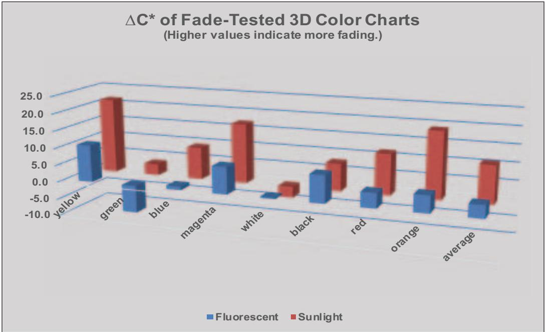
**Figure 5.** Graph of the change in chromaticity (C\*) of color patches exposed to fluorescent light and outdoor sunlight. The samples illuminated with sunlight (red) showed the greatest decrease in chromaticity due to light fading.
