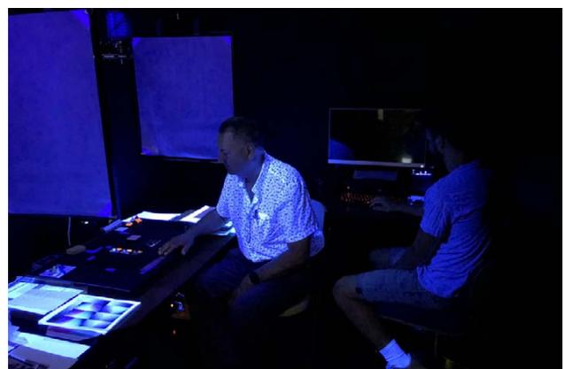
**Figure 7.** Richard Adams (left) and Charles Wilhelm expose the three 3D color targets on the MegaVision EV multispectral camera in order to capture LAB measurements of the color patches. Photos taken with white setup and red, green, and UV exposures.
