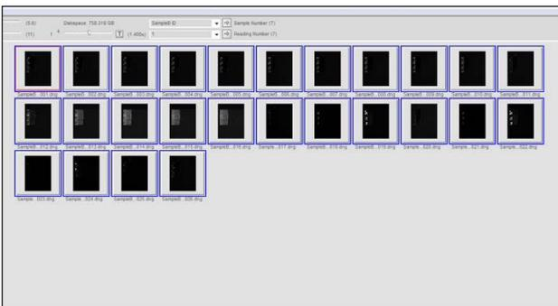
**Figure 9.** Multispectral image capture from the MegaVision EV shows 26 RAW (or DNG format) files captured at wavelengths from 365–1050 nm. With a 50-megapixel monochrome sensor, each capture file is 102 MB, with all 26 files amounting to 2.7 GB. Without the use of the filter wheel, 16 captures total 1.6 GB.
