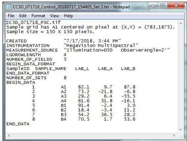
**Figure 10.** This CGATS standard file of LAB color readings is the output of the MegaVision Photoshoot software. The readings correspond to the 8 green rectangles in Figure 7.
