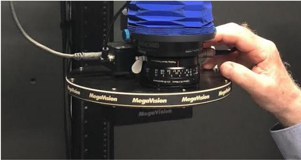
**Figure 12.** A closer view of the MegaVision EV camera showing the filter wheel that can be used to isolate selected wavelengths of illumination in order to quantify degradation of UV-excitation of fluorescing dye and pigment colorants. The filter wheel is also extensively used in the examination of cultural heritage objects.
