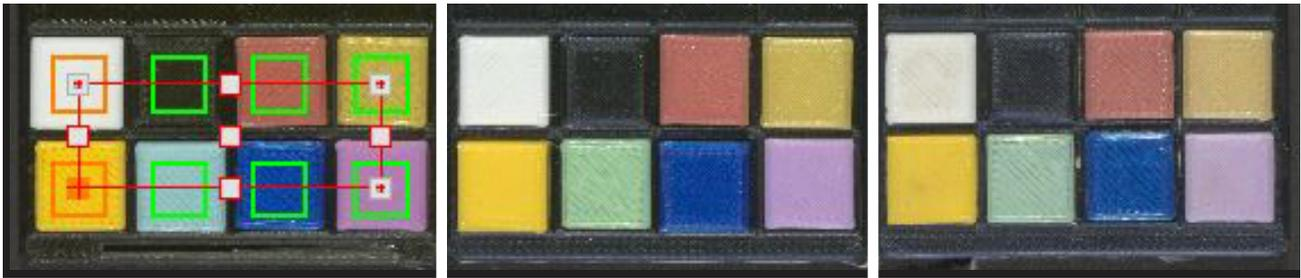
**Photoshoot software measurement screen (green squares are the LAB measurement areas)**
