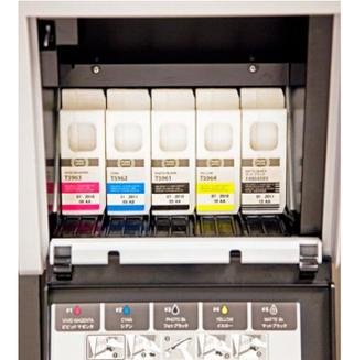
The Epson Stylus Pro 7700 printer employs the same eight-channel piezo print head used in the Epson 7900 and 9900 printers, but by using two ink channels for each of the cyan, magenta, yellow, and black inks, the print speed of the 7700 is twice as fast. The Photo Black and Matte Black inks switch automatically, depending upon the type of paper selected.
