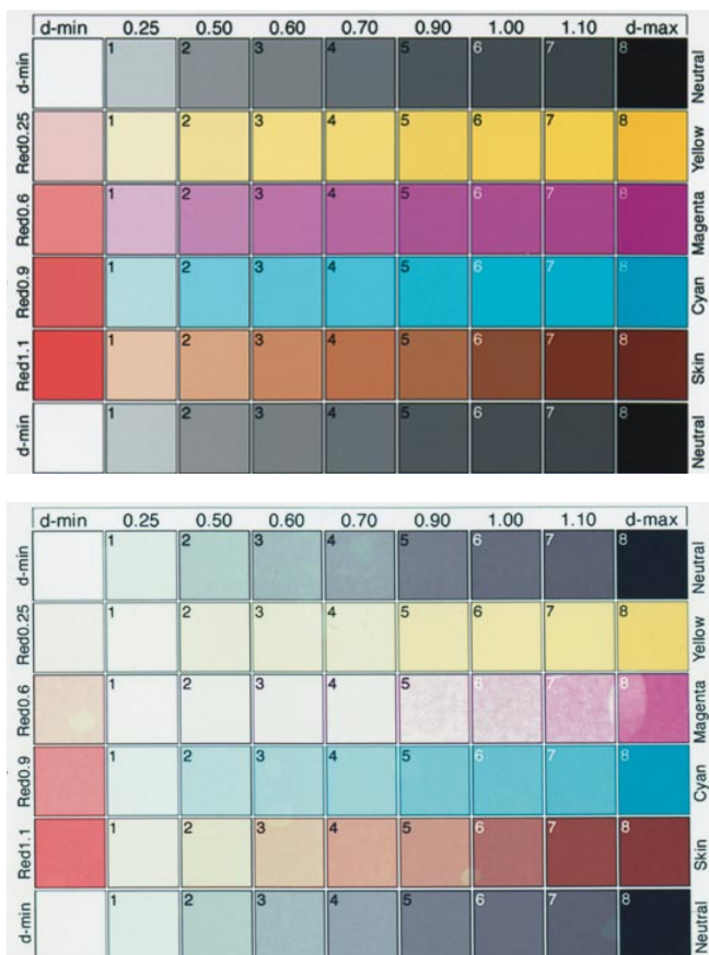
Figure 5. An example of a digitally-printed silver-halide color print which, in the course of an accelerated light/dark cycle glass-filtered xenon arc test (the light/dark cycle is an attempt to compensate for the high black panel temperature and resulting desiccation of the prints under test), the emulsion went above the glass transition temperature and suffered both physical damage (a loss of surface gloss) and an anomalous fading pattern of the magenta dye. The upper print is an unfaded control. Based on both field experience and long-term fluorescent light fading tests, however, it is not anticipated that this type of deterioration would ever occur in real world display conditions. Although glass-filtered xenon arc illumination provides a much better spectral match to indoor daylight filtered through windows than does cool white fluorescent lamps, 13-16 currently available high-intensity xenon test units do not adequately control temperature and relative humidity that photographs encounter in normal home environments. Another drawback of currently available xenon arc units is that because the units normally operate at 80 klux or higher, there are no means available to conduct reciprocity behavior tests at low lux levels (e.g., 1.0 klux). With properly configured light/dark cycles, xenon arc units can provide a good simulation of commercial window display conditions in which prints are exposed to bright sunlight in store windows. But, for realistic simulations of typically encountered indoor display conditions, a properly filtered, "stand-alone" xenon lamp fixture must be used in a temperature and humidity-controlled room with a moderate lux level (e.g., 35 klux), and an air flow adequate to control sample temperature and moisture content (e.g., 24°C and 60% RH).
