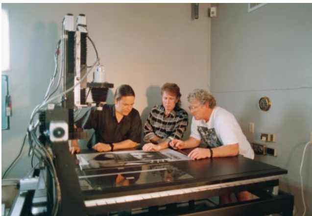
A high-resolution flatbed CCD scanner custom-built by Photometrics, Ltd. was used by Nash Editions to input images from color prints, paintings, and other art work. The scanner could accommodate originals of up to 4x4 feet.
