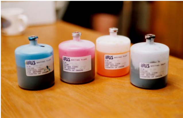
Bottles of the water-base inks employed in the Iris ink jet printers. Initially designed for graphic arts proofing, the standard Iris inks have very poor light fading stability. Inks made with dyes having improved light stability for fine art and photography applications started to become available in 1994.
