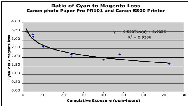
**Figure 6. Ratio of Cyan/Magenta Fade - Canon system.**
