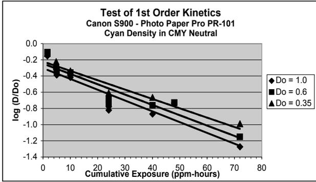
Figure 3. Test of 1<sup>st</sup> order kinetics with Canon System.
