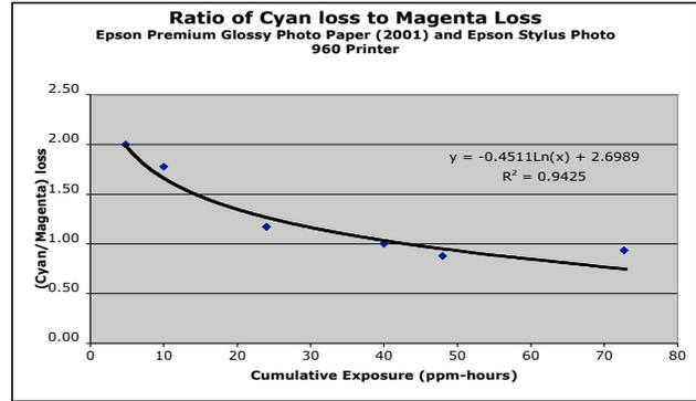
**Figure 7. Ratio of Cyan/Magenta Fade - Epson system**
