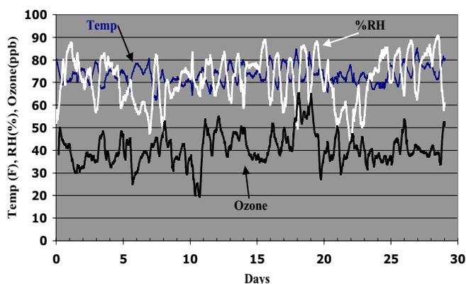
Figure 1. Temperature, relative humidity, and ozone concentrations for an ambient indoor home condition in Boston, July 2004.
