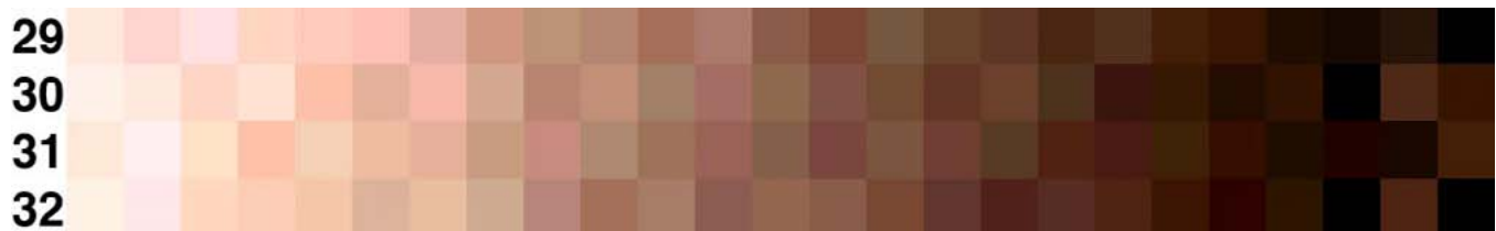
Figure 2. The human skintone colors section of the generic WIR i-Star target consists of 100 patches generated by adjusting the L^* values of the measured LAB values for the “Light Skin” and “Dark Skin” color patches in the Macbeth ColorChecker chart. Photographs of people may range from very high L^* values in specular highlight areas to very low L^* values in deep shadow areas of the face. The number of skintone color patches and neutral/near-neutral patches relative to the total number of patches in the test chart provides a means of weighting these colors in the i-Star analysis. The skintone colors section of the target can also be analyzed separately as an i-Star “Region of Interest.”
