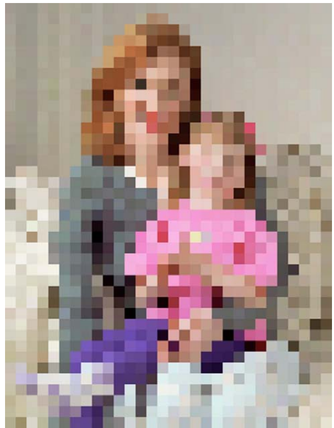
Figure 9. WIR i -Star analysis can be applied to specific images by downsampling and printing to create a measurement test target with pixel blocks that are large enough to be measured with a spectrophotometer. Such image-specific targets are useful for obtaining psychophysical correlations with perceived fading, staining, and changes in color balance in defined classes of images such as professional portraiture, wedding photography, landscape photography, etc.
