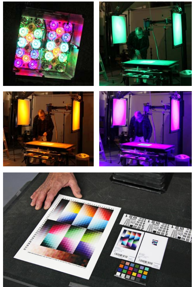
Fig. 2 Illumination from thirteen or more narrow wavelength LED's is used in a darkened room for sequential exposures with the MegaVision camera. Shown above is a standard 800-patch WIR iStar image permanence test target printed on 8.5 x 11-inch photo paper together with two reduced-size “micropatch” WIR iStar test targets.
