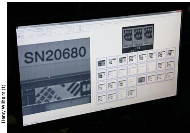
Fig. 5 Software developed by MegaVision handles data collection and analysis of the spectral stacks of the individual monochrome images obtained from exposures at each selected wavelength, and provides a way to compare the spectral data sets from each of the measurements made during the course of an accelerated image permanence test.
