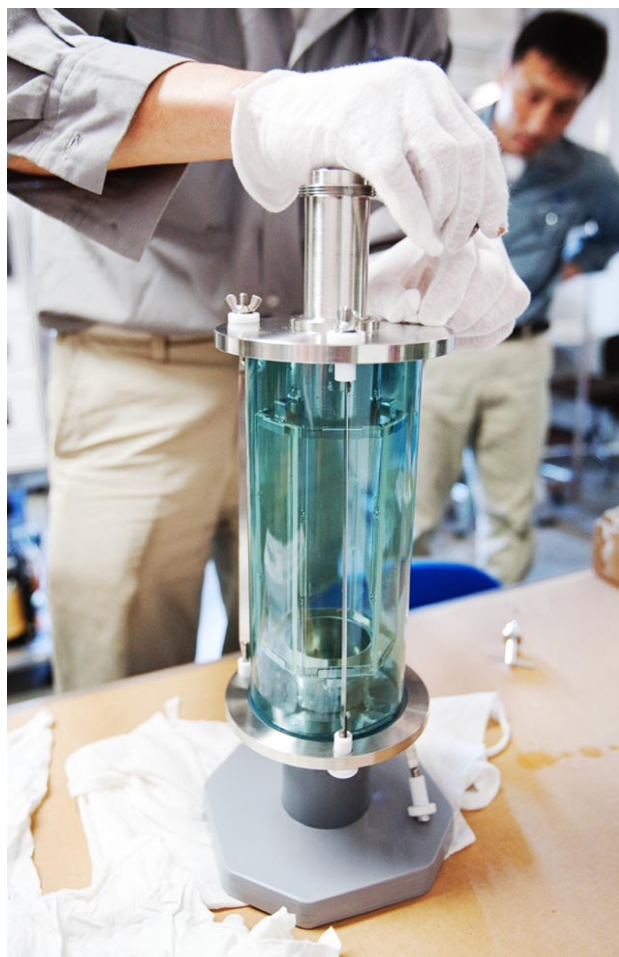
Fig. 6 The water-cooled xenon arc lamp and filter module from the Suga SX75F accelerated test unit. 10 Independent refrigeration systems are provided to cool the lamp as well as to control the air temperature and relative humidity of the test chamber. When operated at 75 klux at the sample plane, the dual IR filters and refrigerated cooling systems are able to maintain a black panel temperature that is only 2°C above the 23°C chamber air temperature (at 50% RH) selected for these tests.
