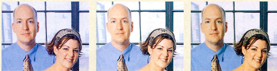
A PRINT MADE using Amazon Imaging inks for the Canon S900 (center) is a bit washed out compared to the one made with Canon inks (left). But a print made with OA100 inks (right) has a yellowish cast.
