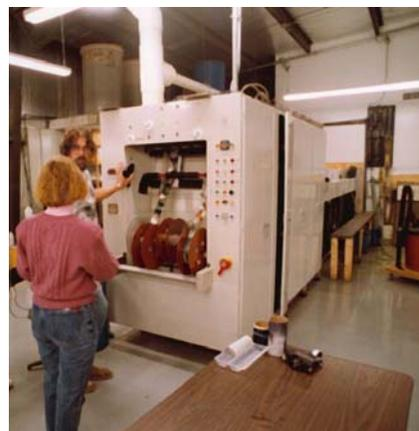
Rolls of exposed paper are processed in a six-strand Agfa RA-4 processor. After cutting, the prints and their negatives are put in customers' envelopes.
