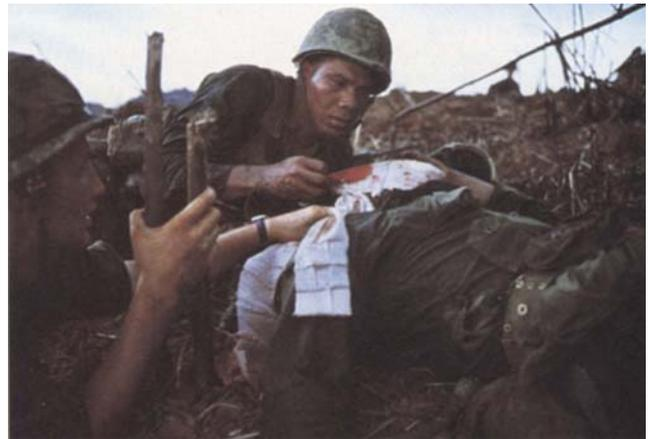
Ilford Cibachrome II (now called Ilfochrome Classic) print, made on a glossy polyester-base, after one year in the accelerated dark fading/staining test. The print showed no detectable fading or staining at the completion of the test (the prints are subject to light fading, however).
