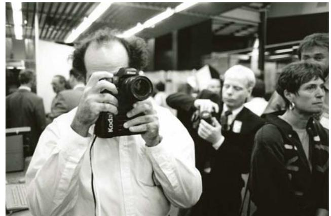
The Kodak Professional DCS 200 Digital Camera is built around a Nikon 35mm autofocus camera body. Instead of film, the camera uses a CCD (charge-coupled device) image sensor; the images are recorded on a small hard disk drive in the base of the camera. Introduced in 1992, the \$10,000 camera is shown here being demonstrated at the Photokina trade show in Germany.
