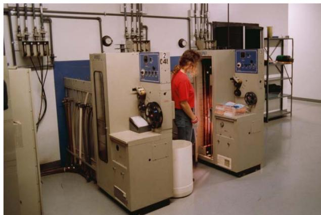
Of the thousands of rolls of film received by the lab each night, about 95 percent are Kodak, Fuji, and other C-41 compatible color negative films in the 35mm and, to a much lesser extent, 110 and 126 formats (Kodak Disc film has almost disappeared from the market). The film is spliced together in long rolls for processing in the machines shown above.
