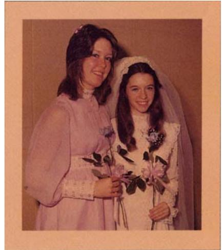
Kodak Ektacolor print after 240 days in accelerated dark fading/staining test.
