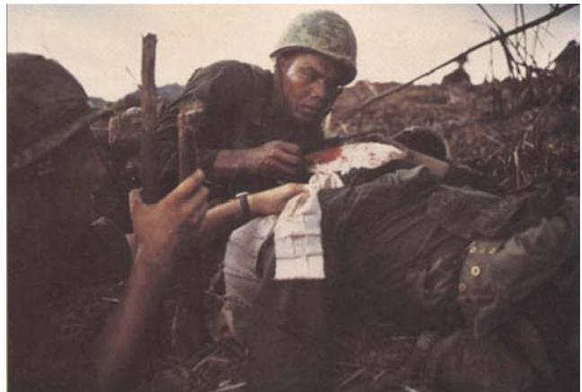
Fujichrome Paper Type 34 RC print (1986–92) after 6 months in the accelerated dark fading/staining test. Fujichrome Paper Type 35 (1992—) has similar stability. Note the low yellowish stain level and the much better cyan dye stability compared with Ektachrome 22 paper.
