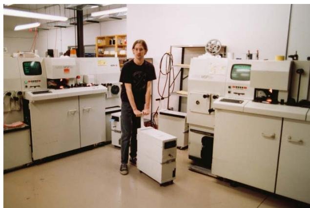
After processing, the spliced rolls of film are printed with Agfa MSP printers. Density and color-balance settings are determined by the computerized printers, each of which can expose between 15,000 and 20,000 prints per hour.
