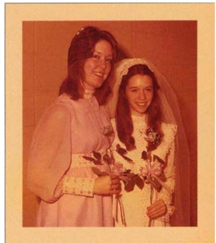
Kodak Ektacolor 74 RC print after 240 days in accelerated dark fading/dark staining test.
