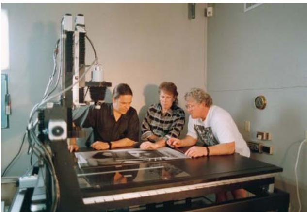
A high-resolution flatbed CCD scanner custom-built by Photometrics, Ltd. is used by Nash Editions to input images from color prints, paintings, and other art work. The scanner can accommodate originals of up to 4x4 feet.
