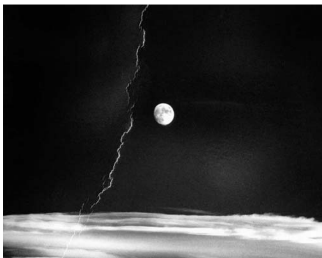
A close-up of a deep crack passing near the moon in the Ansel Adams picture. Had the print not been dry mounted, it might have escaped without damage.
