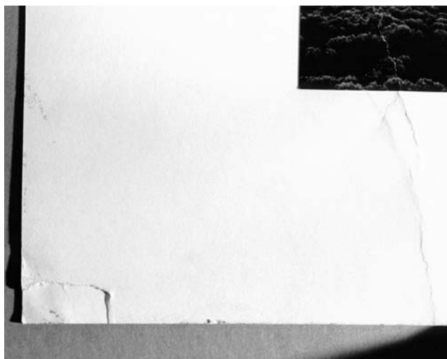
A corner of the mount board was also damaged. Had the print been corner-mounted, it would have been a simple process to remove it and install it in a new mount.
