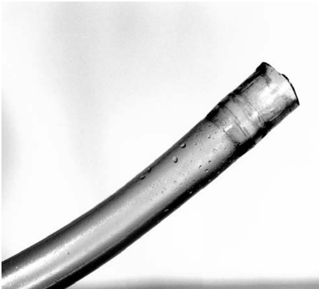
Exudations of plasticizer are not restricted to PVC slide pages, but can occur with many types of heavily plasticized PVC. After about 15 years of storage in this author's darkroom, this PVC hose began to drip plasticizer onto an acrylic plastic film washer.
