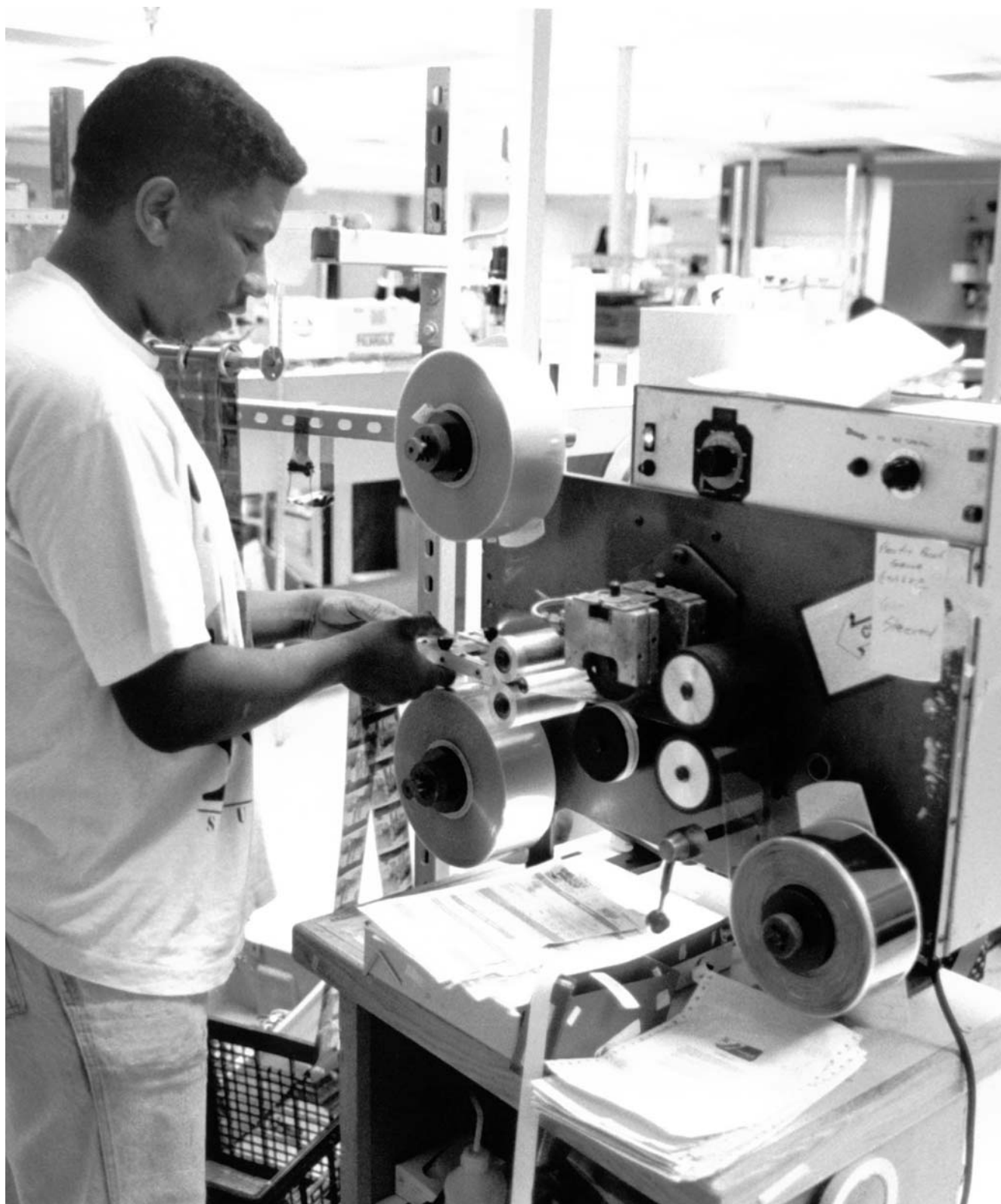
A Photech hot-seal plastic sleeving machine in operation at H&H Color Lab under the watchful eye of Darrell Owens, a film processing technician. H&H, a leading professional portrait and wedding lab located near Kansas City in Raytown, Missouri, processes and proofs up to 2,000 rolls of color negative film a day (mostly in the 120/220 format). Sleeving is done immediately after processing to protect the film from dust and scratches. The film is video analyzed, proofed, and shipped to customers without ever removing the film from the sleeves.
